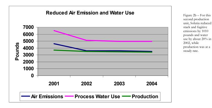
Solutia has also focused its waste reduction efforts on reuse and recycling and associated process changes. For example, in 1992 the plant was an early user of biofilters, which helped reduce air emissions from one unit by over 250,000 lbs per year. Also in the 1990's, Solutia IO substituted less toxic propylene glycol in place of ethylene glycol in many package heat exchange units and modified one of its unit processes to reduce solvent wash volume by 20%.
